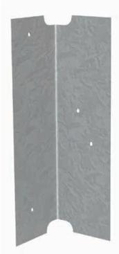
ClarkDietrich EasyClip U-Series clip angles are used to secure U-channel to wall studs for lateral bridging or for miscellaneous rigid connections. U-channel is passed through the stud knockout and an EasyClip U-Series clip is screw-attached or welded to provide a rigid connection. These clips are prepunched for faster, more accurate fastener placement. Do not use in bridging applications when the stud width exceeds 6."
