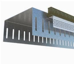
The UltraTRAK slotted system utilizes a UltraTRAK slotted deflection track in conjunction with the UltraBEAD providing a 1 or 2 HR rated assembly for a 3/4" max joint and is UL 2079-Fifth Edition compliant. UltraBEAD creates an easy attachment that is attained with staples through the bead flange. Multiple perforations along the 1-1/8" flange enhance strong compound adhesion and the raised shoulder provides for a flush finish.
