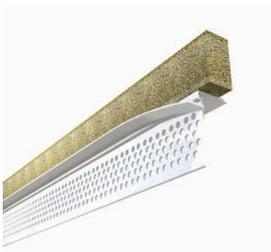
Vinyl L-Bead with compressible foam. UltraBEAD, when used in conjunction with UltraTRAK slotted deflection track or Deep Leg deflection tracks, provides joint protection up to  $\frac{3}{4}$ " for a 1 or 2 HR concrete deck Head of Wall Joint System at 60% compression.
