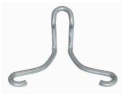
In a ceiling assembly, furring channel clips can be used to suspend U-channel from the overhead structure. Drywall furring channel is commonly clipped or wire-tied perpendicular to the underside of the U-channel at appropriate intervals for screw-attaching drywall.
