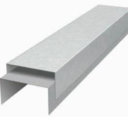
ClarkDietrich DoubleTrack™ system is a two-piece assembly that accommodates deflection of exterior curtain walls. A custom-made deep leg outer track is installed to the underside of the floor deck. A wall assembly is constructed on the floor and slid into place, with a "gap" at the top for deflection. DoubleTrack deflection assemblies cannot be used in axial load-bearing stud conditions or above continuous window spandrels.
