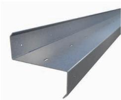
ClarkDietrich Z-Girt is used as a primary rainscreen framing component with depths matching common exterior insulation thicknesses while providing a uniform plane for cladding attachment. It can be installed in a horizontal or vertical orientation. The type of fastener and spacing will vary based on application.
