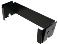
The YurClip is used in combination with deep leg deflection track. Saving labor time, they do not require screws in the stud or bridging installed continuously throughout the upper most punchouts. YurClips can be installed on the deflection track or on the stud first. Adjustable for layout errors or changes. Wall studs work in clip either way.
