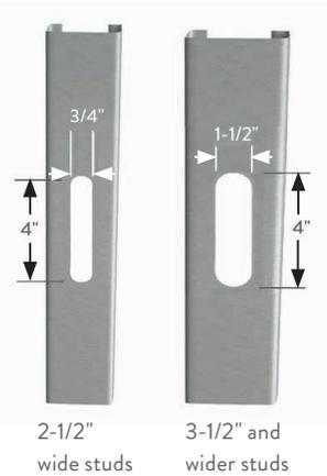
ClarkDietrich cold-formed C-studs for axial load-bearing and curtain wall framing are prepunched with knockouts at regular intervals. These punchouts are specifically designed to allow for rapid installation of pipes, electrical conduit and wall bridging.
