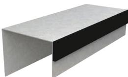
Profile with two solid legs with fire stop on one side. Composite fire stop/framing for use in up to three-hour fire-rated shaft wall assemblies. Provides joint protection for up to 1" overall movement with UL 2079 Class II or III Movement Capabilities. Minimum CP60 coating. One leg (front) having intumescent per listed assemblies in UL Fire Resistance Directory.
