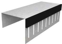
Profile with one slotted leg and one solid leg with fire stop on slotted side. Composite fire stop/framing for use in fire-rated wall assemblies. Provides joint protection for up to 1" overall movement with UL 2079 Class II or III Movement Capabilities. Minimum CP60 coating. One leg with slots spaced 1" o.c. for positive attachment of studs per listed assemblies in UL Fire Resistance Directory.
