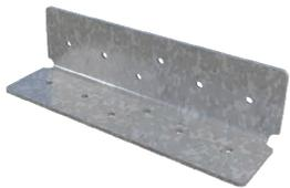
SwiftClip LS-Series™ support clips are used in multiple construction projects, specifically in conjunction with studs and track. The L-shaped clips fit between the stud flanges, so that shorter length clips do not need to be ordered. These labor time-savers include prepunched holes for quicker screw attachments, and are punched to accommodate for U-channel lateral bracing connections.
