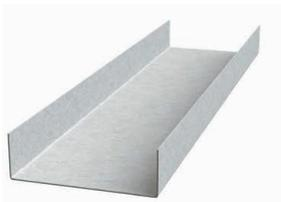
ClarkDietrich structural track is a U-shaped framing component used as top and bottom runners to secure wall studs. Structural track is also used as end support closures for joists at exterior or foundation walls, head and sill plates of wall openings and solid blocking. Track is normally ordered in corresponding size and gauge to the wall studs.
