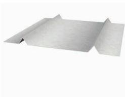
Corrugated strap for horizontal use to span fluted areas of unprotected or protected metal decks in up to 2 hr rated assemblies. Profile attached to fluted deck max 16" o.c. on both sides.
