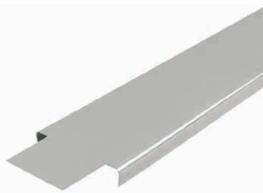
Katz™ bridging maintains accurate member spacing to prevent bowing or flexing of nonload-bearing framing. It can also be used as backing between studs in areas where cabinets or fixtures are to be attached. Use standard 24" o.c. frame spacing.
