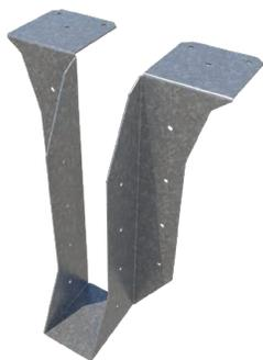
Bridle hangers are commonly used to attach cold-formed C-joists to structural steel beams, wood ledgers or masonry block. Connections can be made with screws, powder-actuated fasteners, drill-in concrete anchors or welding. Single- and double-wide hangers are also available in other widths and depths. The MB hanger can also be sloped to a maximum of 45°. Skew only: MB series can be skewed to a maximum of 45°—maximum allowable download is 62% of table load.
