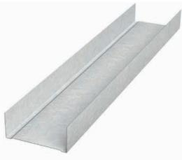
ClarkDietrich C-runner (or H-track) is used to secure H-stud and gypsum shaftliner panels in area separation wall assemblies. Attached to the foundation with powder-actuated fasteners, C-runner is also used as top track to cap the H-stud and gypsum shaftliner panels, with a second track screwed back-to-back to the lower runner, to hold the next assembly level.
