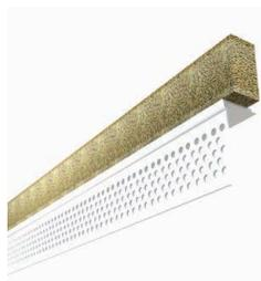
Vinyl L-Bead with compressible foam. UltraBEAD, when used in conjunction with UltraTRAK slotted deflection track or Deep Leg deflection tracks, provides joint protection up to 3/4" for a 1 or 2 HR concrete deck Head of Wall Joint System at 60% compression.
