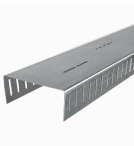
MaxTrak 2D is a head-of-wall deflection track that is used for framing exterior curtain walls and nonload-bearing interior walls where vertical deflection and horizontal drift occurs—and serves as a connecting member that isolates the cold-formed steel framing system from the movement of the primary structure.
