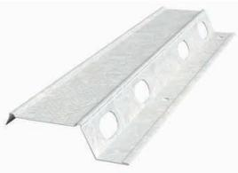
Made of 25 gauge steel, RC-1 Pro is used as a cross-furring member for resilient attachment of gypsum. Knurled face makes wallboard application easier.
