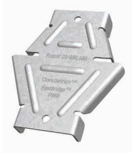
The ClarkDietrich FastBridge™ Clip is used to secure 1-1/2" U-channel (or Cold Rolled Channel-(CRC)) to structural wall studs when used in load-bearing or curtain wall applications. The wall stud friction fit design allows for as little as one screw for the connection to the U-channel. Do not use in studs over 8" wide.
