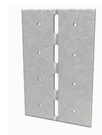
ClarkDietrich Skewable Angles are used to make rigid attachments of joist-to-joist or joist-to-other-miscellaneous framing. This clip is ideal for making off-angle connections. It is easily field bent from 0° to 135°.
