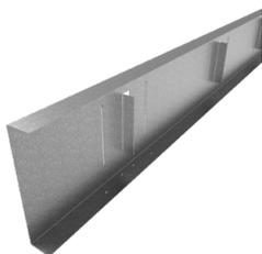
Another major component of the TradeReady floor system, the standard 12'-long rim drastically reduces framing time and effort. Rims have pre-formed, prepunched attachment tabs at 12", 16", 19.2" or 24" o.c. spacing to eliminate layout time—and ensure fast, proper fastener placement. Embossed stiffening ribs on each side of the tabs provide additional reinforcement, for a significant reduction of web stiffeners (squash blocks) and support clips in a majority of applications.
