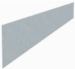
ClarkDietrich backing plate is a general multipurpose flat stock that is used for backer plate to support shelves, cabinets, fixtures or handrails when applied to metal framing. **Backing plate should not be used as tension strapping or cross bracing.** Commercial Strapping should be used in those applications.
