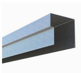
BlazeFrame RipTRAK Shaftwall is a ceiling runner with an offset shoulder that represents the thickness of the wall material (5/8" or 1-1/4"). A second piece of board/wall material is fit flush to the fluted deck or slab and is then attached to the shoulder. The BlazeFrame RipTRAK Shaftwall is a UL tested fire-rated head-of-wall joint system for up to 4" Total Deflection Movement.
