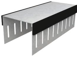
Profile with two slotted legs with fire stop on both sides. Composite fire stop/framing for use in fire-rated wall assemblies. Provides joint protection for up to 1" overall movement with UL 2079 Class II or III Movement Capabilities. Minimum CP60 coating. Legs with slots spaced 1" o.c. for positive attachment of studs per listed assemblies in UL Fire Resistance Directory.
