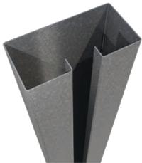
As part of the HDS Framing System, the jamb stud eliminates capped members, allowing drywall screws to drive through only one thickness of material. All material is CP60.
