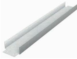
The third component of the TradeReady® Floor System, TradeReady Structural Bridging is pre-cut to fit securely between the underside of the floor joists to prevent joist rotation. Prepunched for quick attachment, it's an economical alternative to cross bracing, X-bracing or strapping. For easy attachment, install continuous row of blocking every 8' o.c. maximum, and staggered.
