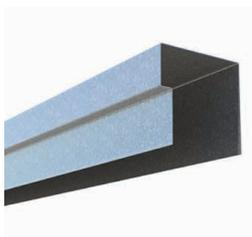
BlazeFrame RipTRAK Shaftwall is a ceiling runner with an offset shoulder that represents the thickness of the wall material (5/8" or 1-1/4"). A second piece of board/wall material is fit flush to the fluted deck or slab and is then attached to the shoulder. The BlazeFrame RipTRAK Shaftwall is a UL tested fire-rated head-of-wall joint system for up to 4" Total Deflection Movement.
