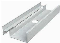
Engineered to maintain shaftwall integrity, ClarkDietrich C-T cavity shaftwall studs are punched with 1" circular knockouts at 12" o.c. for easy installation of conduit or other mechanical service lines.
