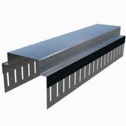
Profile with two slotted lower legs with firestop on both sides. Composite Firestop Deflection Track System with "offset step" accommodates fireproofing up to 1-1/2" thick in head of wall and wall to wall (column) assemblies. Two legs with slots spaced 1" o.c. for positive attachment of studs.
