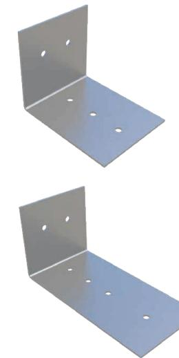
ClarkDietrich aluminum burn clips are used as part of the H-stud area separation wall assembly and are designed to melt when exposed to fire. The clips hold the area separation wall assemblies in place at the floor, roof and truss line between adjacent units. In a fire, the aluminum burn clips on the fire-ridden side of the wall will melt, allowing the wall structure for that side to collapse.
