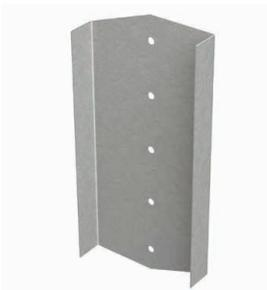
EasyClip™ QuickTwist™ web stiffeners are used to provide reinforcement of joist webs to prevent crippling. Web reinforcement is often required by design to enhance the load capacity of joists. The unique design of QuickTwist allows the installer to insert the stiffener on the inside of the joist *after* the joist is installed. This stiffener eliminates the need to pre-insert traditional web stiffeners prior to joist installation. The one-piece assembly is easily rotated in place for a tight fit.
