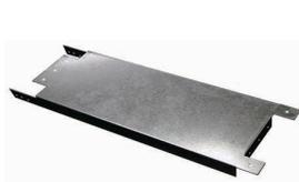
The ClarkDietrich Backer Bar was specifically designed to meet the demand for the attachment of multiple items and heavier items to interior partitions. Provides superior connection shear and pullout strength for handrails, shelves and other wall fixtures. Designed, tested and patented by Bailey®. Manufactured and distributed in the USA by ClarkDietrich®.
