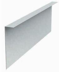
ClarkDietrich L-headers are prefabricated, cold-formed 90° L-sections that are used in load-bearing wall framing. They slide easily into place and eliminate the labor-intensive process of built-up field-assembled headers. Install as single, one header one side, or double, two headers, one on both sides.
