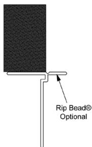
BlazeFrame® Perimeter L-Bead creates an easy attachment that is attained with staples through the bead flange. Multiple perforations along the 1-1/8" flange enhance strong compound adhesion and the raised shoulder provides for a flush finish. Rigid vinyl is rust proof, dent resistant and easy to field cut without distorting profile or leaving sharp edges and burrs.
