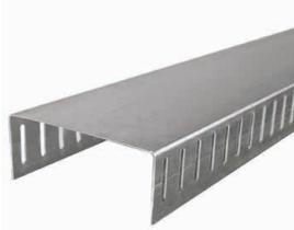
MaxTrak® is a head-of-wall deflection track that is used for framing exterior curtain walls and nonload-bearing interior walls where vertical deflection occurs—and serves as a connecting member that isolates the cold-formed steel framing system from the movement of the primary structure.
