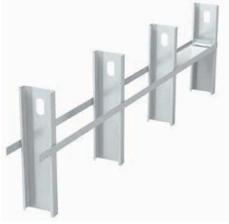
Properly spaced horizontal steel bracing provides resistance to stud rotation and minor axis buckling under wind and axial loads. Block and strapping is typically used when wall studs exceed 6". Field cut, blocking is used if knockouts do not align. It's also used as bridging when framing members are unpunched.
