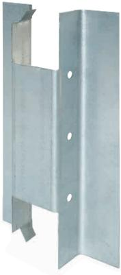
The FastBack® backing system features a universal design that works with studs in either direction—concealing fasteners on the face of the product. The system creates an interlocked design between the stud and track for baseboard backing installations; and a cutaway design allows backing and bracing to be installed all the way to the floor.
