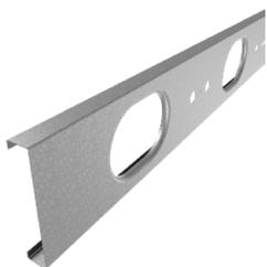
ClarkDietrich TradeReady® steel joists meet the requirements of most typical building layout and floor/roof loads. Large extruded holes (spaced at 24" o.c.) accommodate HVAC, mechanical, plumbing, electrical and sprinkler runs. The joist also features a series of smaller holes for electrical and technology lines. Hole sizes range from 4-1/4" oval to 10" round, based on member depth.
