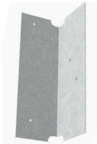
ClarkDietrich EasyClip X-Series™ clip angles are used to secure U-channel to wall studs for lateral bridging. U-Channel is passed through the stud knockout and an EasyClip X-Series clip is screw-attached or welded to provide a rigid connection. X-Series clip angles and U-channel should not be used in lateral bridging when stud width exceeds 6."
