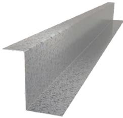
ClarkDietrich Z-furring is used to furr out interior masonry or poured concrete wall substrates and to support rigid polystyrene, mineral, or fiberglass batt insulation while providing a uniform plane for gypsum panel attachment. Z-furring should be installed vertically with the 3/4" flange against the substrate. The type of fastener and spacing will vary based on application. Install gypsum wallboard parallel or perpendicular to Z-furring.
