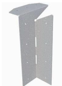
The Universal Joist Hanger is used to connect joists to CFS headers (with screws, welds or PAF fasteners) and steel I-beams (with welds or PAF fasteners). The UJH is sized to fit joist sizes from 8" to 14" deep.
